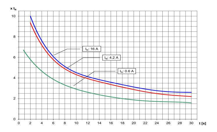
Our wire-wound tubular resistors type FW can be highly overloaded for a short time. This overload behaviour is shown in the curves above. The overload factor in function of the time is shown for three different nominal currents  $I_N$ . The intermediate values of the nominal currents can be interpolated or extrapolated. The curves show standard values without high accuracy.
