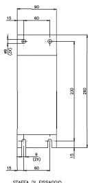
STAFFA DI FISSAGGIO MOUNTING PLATE
