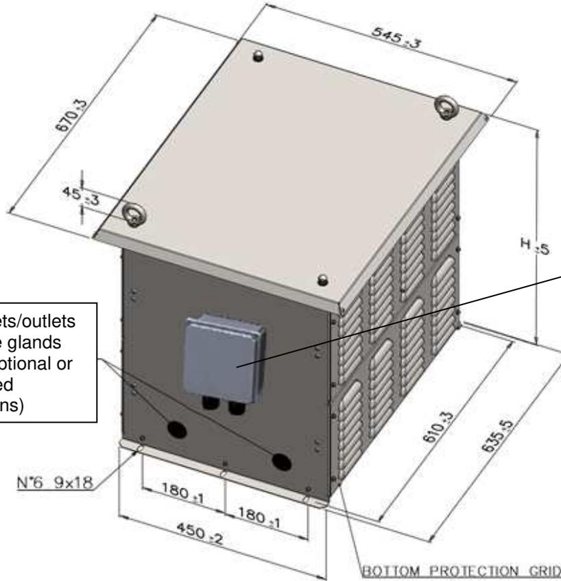
Cable inlets/outlets with cable glands 2xM25 (optional or customized connections)
