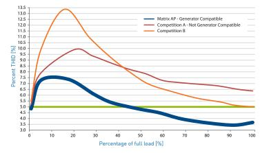
Matrix AP Harmonic Filters can help ensure that your system meets the IEEE-519 requirements for harmonic current.
